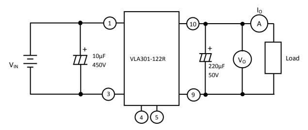
It is used the electrolytic capacitors which has the low impedance for output capacitor.
