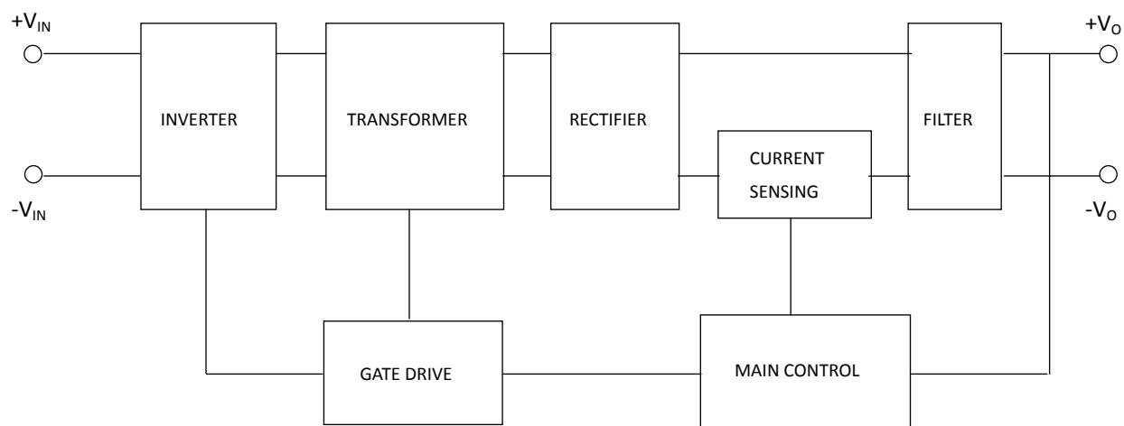
**ISOLATED TYPE DC-DC CONVERTER**
